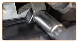
Tighten the thermostat housing fasteners. Use a drive socket #10. Use a torque wrench. Tighten it to 7 nm torque.
