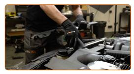
Unscrew the coolant reservoir cap.
