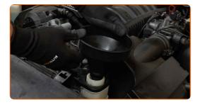
Pour coolant in the coolant reservoir.
