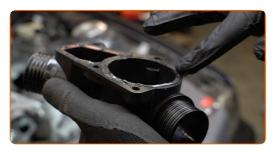
23 Install the new thermostat housing.
