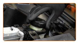
Screw on the coolant reservoir cap.
