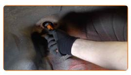
Place the shock absorber in the wheel arch and secure it.
