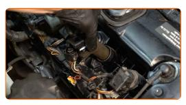
Plug in the ignition coil connector.
