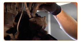
Install the brake caliper retaining spring.
