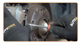
Remove the brake caliper.
