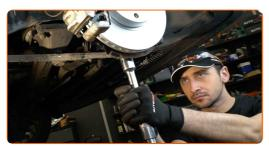
Tighten the fastener connecting the stabilizer bar with the control arm. Use a combination spanner #17. Use a drive socket #17. Use a torque wrench. Tighten it to 42 Nm torque.
