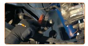
Unscrew the fastener connecting the stabilizer bar with the control arm. Use a combination spanner #13. Use a drive socket #13. Use a ratchet wrench.
