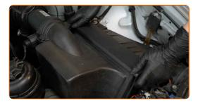
Remove the air filter housing.
