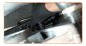
Loosen the clamps of the coolant hoses. Use a drive socket #7. Use a ratchet wrench.
