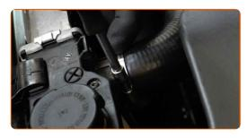
Remove the coolant reservoir cap.
