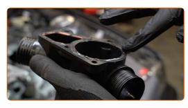
23 Install the new thermostat housing.
