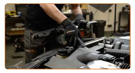
5 Unscrew the coolant reservoir cap.
