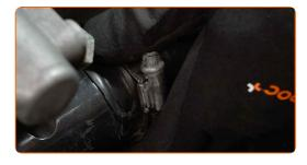
Loosen the coolant hose clamp. Use a drive socket #7. Use a ratchet wrench.
