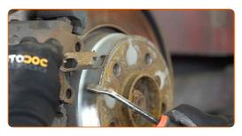
Remove the brake caliper.
