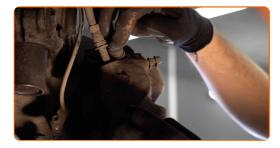
Install the brake caliper retaining spring.
