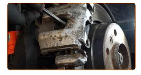
Remove the brake caliper.
