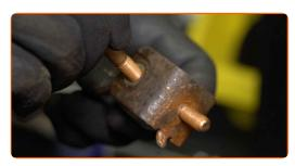
Screw in the fastener of the stabiliser link bracket. Use a drive socket #13. Use a ratchet wrench.
