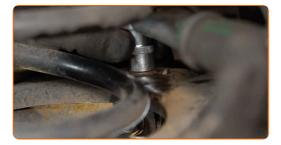
Tighten the fastener of the stabiliser link bracket. Use a combination spanner #13. Use a drive socket #13. Use a torque wrench. Tighten it to 25 Nm torque.
