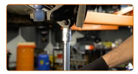
Tighten the fastener connecting the stabilizer bar with the control arm. Use a drive socket #13. Use a torque wrench. Tighten it to 27 Nm torque.
