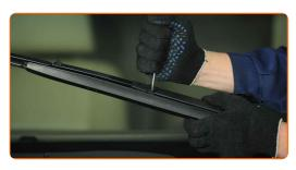
Remove the blade from the wiper arm.
