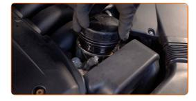
Install a new oil filter housing cover and tighten it. Use the 86-16F socket. Use a torque wrench. Tighten it to 25 Nm torque.
