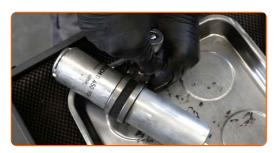
Remove the fuel filter fastening bracket.
