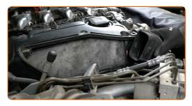
Undo the fastening screws of the air filter cover. Use HEX No.H5. Use a ratchet wrench.
