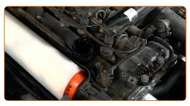
Reinstall the air filter cover. Fasten it.
