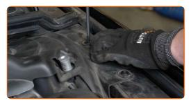
Remove the protective caps out of the shock absorber mounting fastener.
