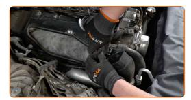
Unscrew the fasteners of the back section of the engine cover. Use HEX No.H5. Use a ratchet wrench.
