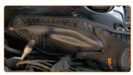
Screw in the fastener of the air intake pipe. Use HEX No.H5. Use a ratchet wrench.
