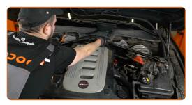
Screw in the fasteners of the diagonal braces. Use Torx T40. Use a ratchet wrench.
