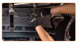
Remove the fender protection cover.
