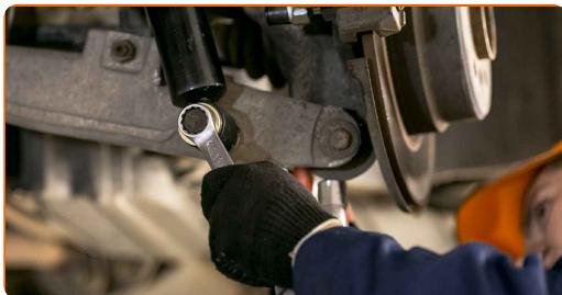
**45** Treat the shock absorber fasteners. Use copper grease.
