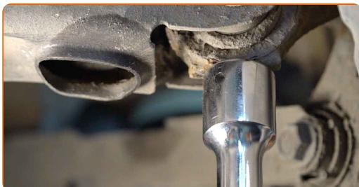
**42** Attach the lower part of the shock absorber.
