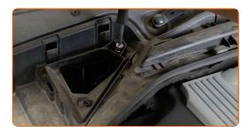
Remove the bottom part of the cabin filter housing.
