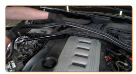
Unscrew the fasteners of the bottom part of the cabin filter housing. Use a drive socket #13. Use a ratchet wrench.
