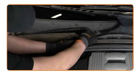
Unscrew the fasteners of the cabin filter housing cover. Use a drive socket #13. Use a ratchet wrench.
