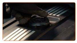
Unscrew the filter housing cap together with the old filter element. Use the 86-16F socket. Use a ratchet wrench.
