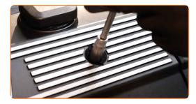
Install the engine cover and secure it.
