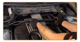
9 Remove the cabin air filter housing.
