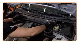
Screw in the fasteners of the cabin filter housing cover.
