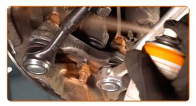
Tighten the rod end fastening. Use a drive socket #16. Use a torque wrench. Tighten it to 40 nm torque.
