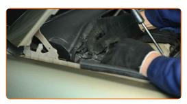
Tighten the fasteners of the cowl grille. Use a drive socket #8. Use a torque wrench. Tighten it to 11 nm torque.
