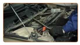
Screw in the fasteners of the diagonal braces.
