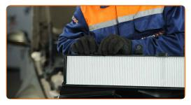
Reinstall the cabin filter housing cover.
