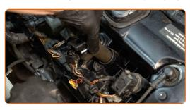
Plug in the ignition coil connector.
