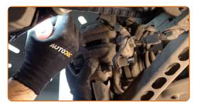
Remove the brake caliper.
