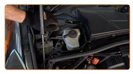
Unscrew the brake fluid reservoir cap.
