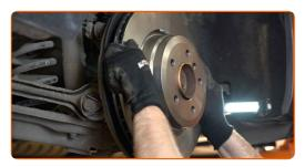
Tighten the brake disc fastening. Use HEX No.H5. Use a torque wrench. Tighten it to 16 Nm torque.
