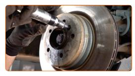
Remove the brake disc.
