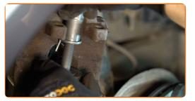
30 Treat the brake pads in the area where their surface comes into contact with the brake caliper bracket. Use antisqueal paste.
