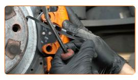
Remove the brake caliper.
