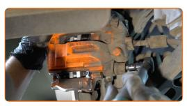
23 Install the dust boot caps of the brake caliper guide pins.
