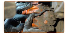
Install the brake caliper retaining spring.
