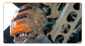
Connect the brake pads wear sensor.
