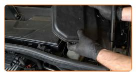
Unscrew the brake fluid reservoir cap.
