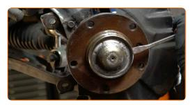
Unstake the wheel hub retaining nut. Use a flat metal-working chisel. Use a hammer.
