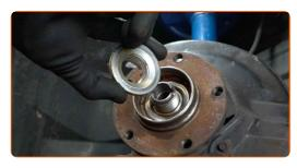
Remove the wheel hub together with the bearing. Use 3-Arm Gear Puller.
