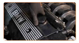
Screw in the engine cover fasteners. Use a drive socket #10. Use a ratchet wrench.
