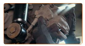
Connect the brake pads wear sensor. Use round-nose pliers.
