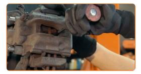
Remove the brake caliper.
