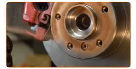
Clean the brake disk surface. Use a brake cleaner.
