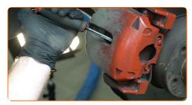
Detach the brake caliper retaining spring. Use a crowbar.
