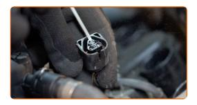
Install the ignition coils to the spark plug wells. Make sure you hear a click indicating that it is locked in place.
