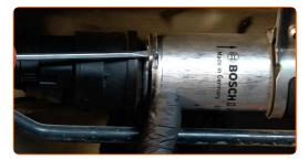
Loosen the fastening clamp of the fuel filter pipe. Use a flat screwdriver.
