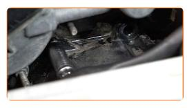
18 Remove the thermostat housing.
