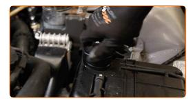
Install the engine cover and secure it.
