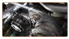
Pull aside the V-ribbed belt tensioner pulley. Use a combination spanner #26.
