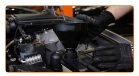
Pour coolant in the coolant reservoir.
