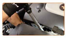
51 Install the fan shroud clips.
