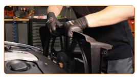
Unscrew the engine cover fastener. Use HEX No.H5. Use a ratchet wrench.
