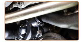
Tighten the coolant hose fastener. Use a drive socket #10. Use a torque wrench. Tighten it to 6 nm torque.
