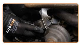
Treat the thermostat housing mounting seat. Use a sealant.
