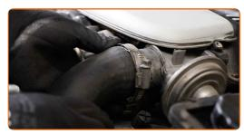
Screw in the intercooler hose clamp. Use a drive socket #7. Use a ratchet wrench.
