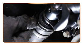
Clean the mounting seats of the V-ribbed belt. Use all-purpose cleaning spray.
