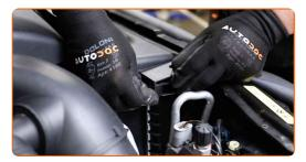
Open the coolant system bleed screw. Use a flat screwdriver.
