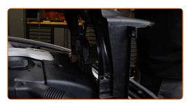
Tighten the cooling fan fastener. Use a combination spanner #32 (2 pieces). Use a torque wrench. Tighten it to 33 Nm torque.
