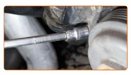
Remove the thermostat housing. Use a crowbar.
