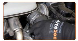
Unscrew the fastener of the coolant hose clamp. Use a drive socket #10. Use a ratchet wrench.
