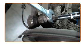
Unscrew the arm fastening to the beam. Use a combination spanner #16.
