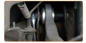
Tighten the arm fastening to the beam. Use a drive socket #16. Use a torque wrench. Tighten it to 110 nm torque.
