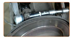
Screw in the fastener connecting the control arm to the subframe. Use a combination spanner #16.
