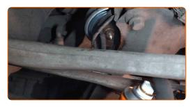
Remove the fender protection cover.
