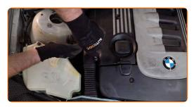
Detach the air duct housing from the air filter housing.
