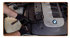
Unscrew the upper fastener of the engine mount. Use a drive socket #16. Use a ratchet wrench.
