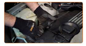
Secure the fastener of the air intake duct. Use HEX No.H5. Use a ratchet wrench.
