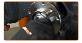
Tighten the wheel hub nut. Use a drive socket #46. Use a torque wrench. Tighten it to 290 Nm torque.
