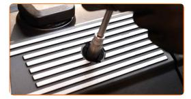
Install the engine cover and secure it.
