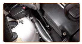
Support the engine in the oil pan area. Use a hydraulic transmission jack.
