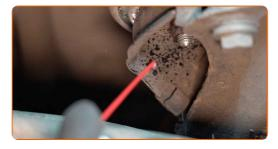
Unscrew the lower fastener of the engine mount. Use a drive socket #16.
