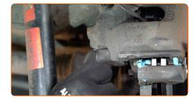
Install the brake caliper retaining spring.
