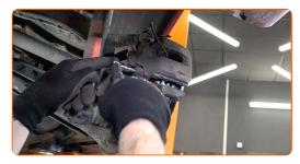
20 Install the dust boot caps of the brake caliper guide pins.
