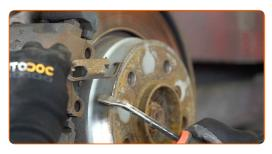
Remove the brake caliper.
