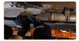
Detach the fuel pressure regulator from the fuel filter. Use a crowbar.
