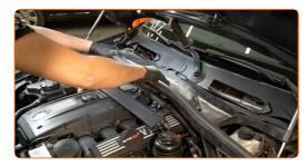
Screw in the fasteners of the lower part of the scuttle panel. Use a drive socket #8. Use a ratchet wrench.
