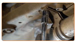
Disconnect the fuel supply lines from the fuel filter.
