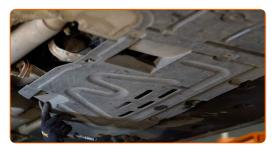
Tighten fixing bolts of the protective cover. Use a drive socket #8. Use a ratchet wrench.
