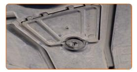
Screw in the fastener of the drain plug access panel. Use a flat screwdriver.
