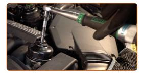
Remove the oil filler cap. Insert the funnel.
