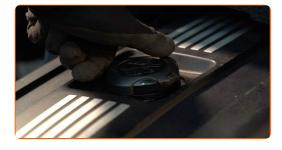
Unscrew the filter housing cap together with the old filter element. Use the 86-16F socket. Use a ratchet wrench.
