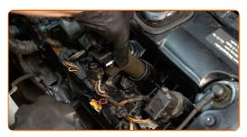
Plug in the ignition coil connector.
