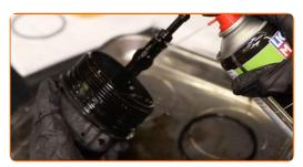
Install a new O-ring to its mounting seat on the filter cover.
