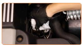
Install the cover of the oil filter housing and screw it on. Use a drive socket #36. Use a torque wrench. Tighten it to 25 Nm torque.
